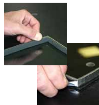
Poor Tape Application Quality
